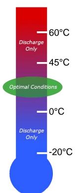
At temperatures above 60°C, the battery must **NOT** be **operated** (charge or loads). Please move the battery into a cooler environment.
