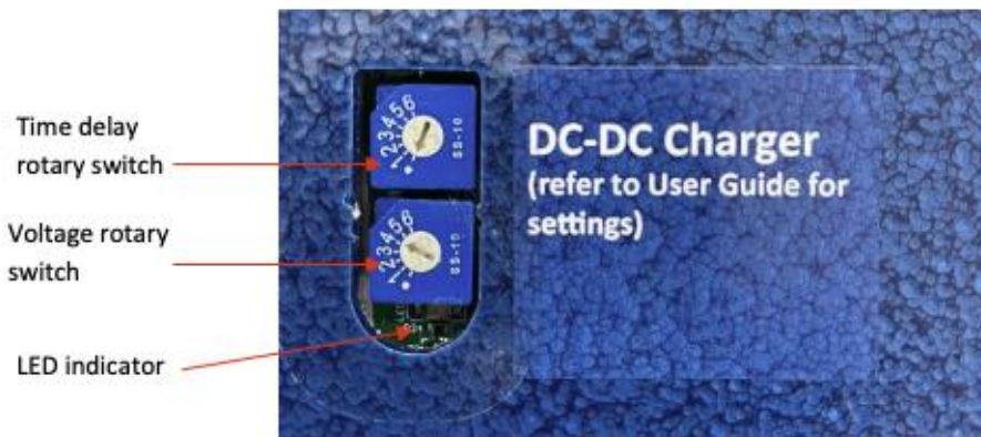
Figure 12: DC-DC Charger switches
