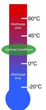
At temperatures above 60°C, the battery must **NOT** be **operated** (charge or loads). Please move the battery into a cooler environment.
